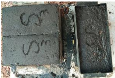
Moulding of soil-organic waste
